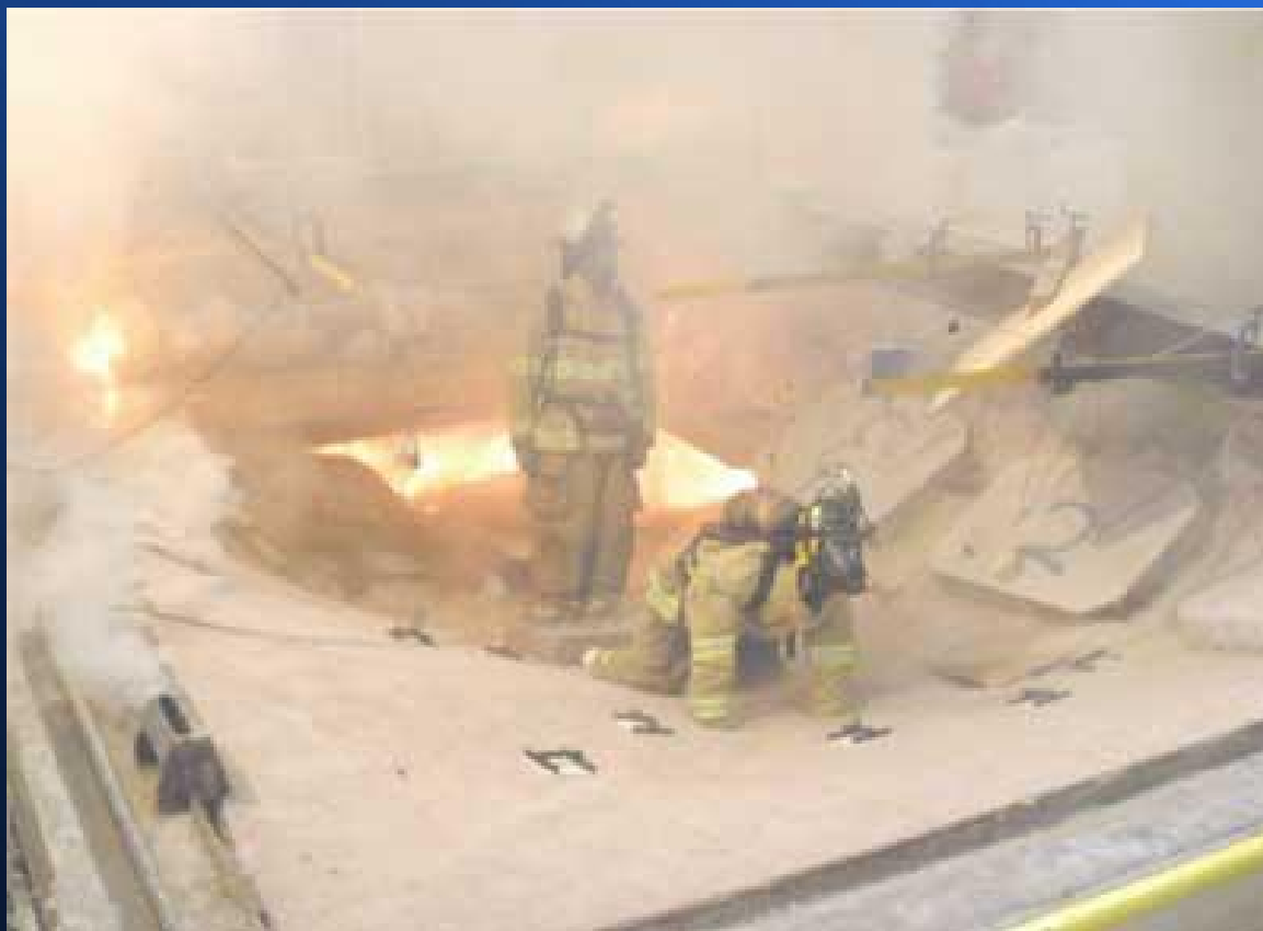
Floor Colapse In as Little as 6 Minutes.
